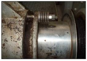
Chesterton's 5150 Rotary Live Loading system avoids leakage by automatically maintaining the correct sealing force on the packing set.
